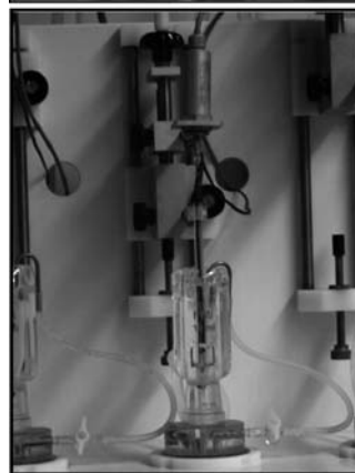
Fig. 1 Photograph of the Schuler organ bath FMI IOA-5301. The system consists of eight single organ bath units that enable simultaneous measurements. A single organ bath chamber is depicted to present the set-up: The arterial ring is placed inside the perfused chamber inbetween two stainless high-grade steel hooks, linked to the transducer. The output of the transducer is connected to the amplifier. The pre-tension of the renal artery ring is adjusted manually to 2 g at the pre-adjustment screw. The circumferential contractions of the rings are registered and stored digitally on a PC
